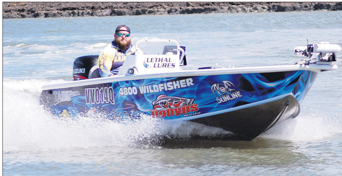
The Wildfisher not only does around 75km/h, it also does it drier than most boats thanks to some sizable spray chines.
