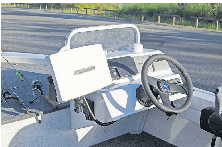
The side console fixed to the front casting deck is a great space-saver. Note Col's Humminbird sounder that can be turned for use while fishing from bow or stern.
